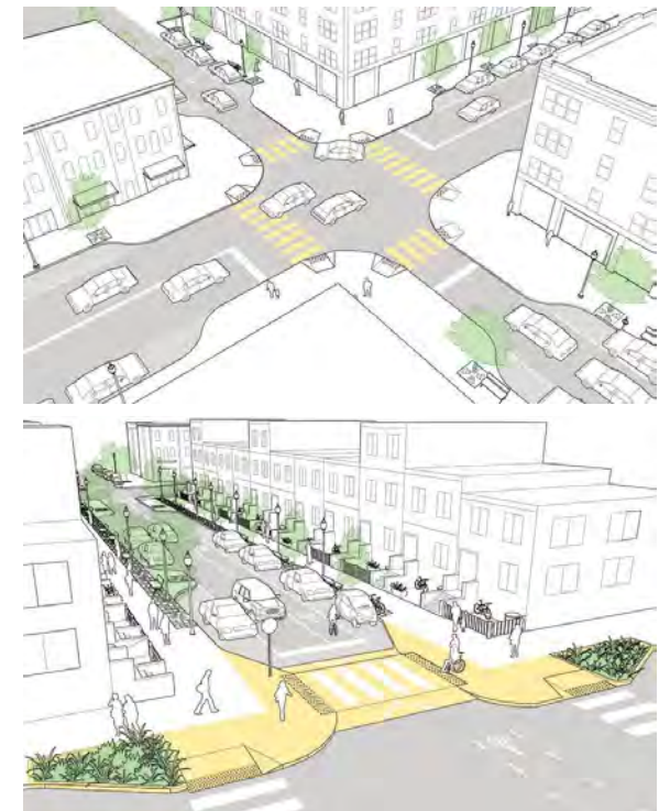
Figure 11: Pedestrian Bulbout & High-visibility Crosswalk Treatment Examples
